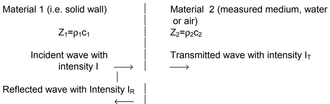
In most cases we are only able to measure the reflected wave and not the transmitted (this will be disturbed during propagation in unknown medium). This is the reason, why it is normally necessary to know the impedance of the solid wall. But it is also possible to measure it using air as reference medium (material 2). In this case the measurement would need following steps:
