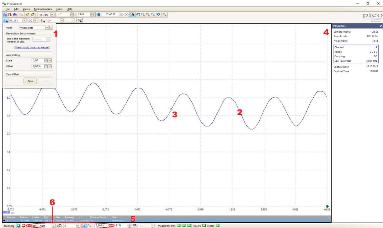
Figure 3. Main screen from oscilloscope software (PICO OSCILLOSCOPE).
