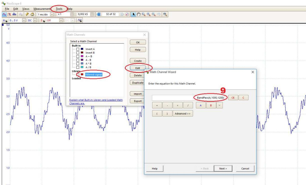
Figure 5. Setting up a digital filter
