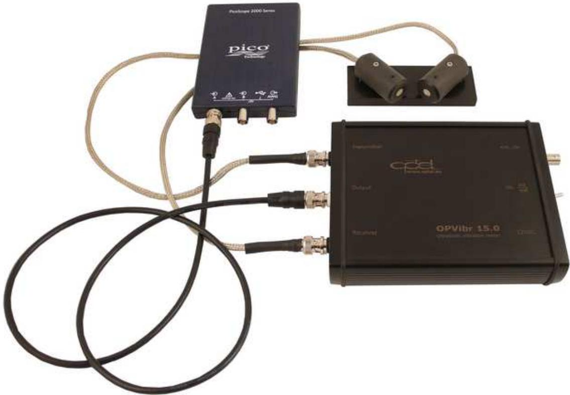
Figure 1. Ultrasonic measurement system
