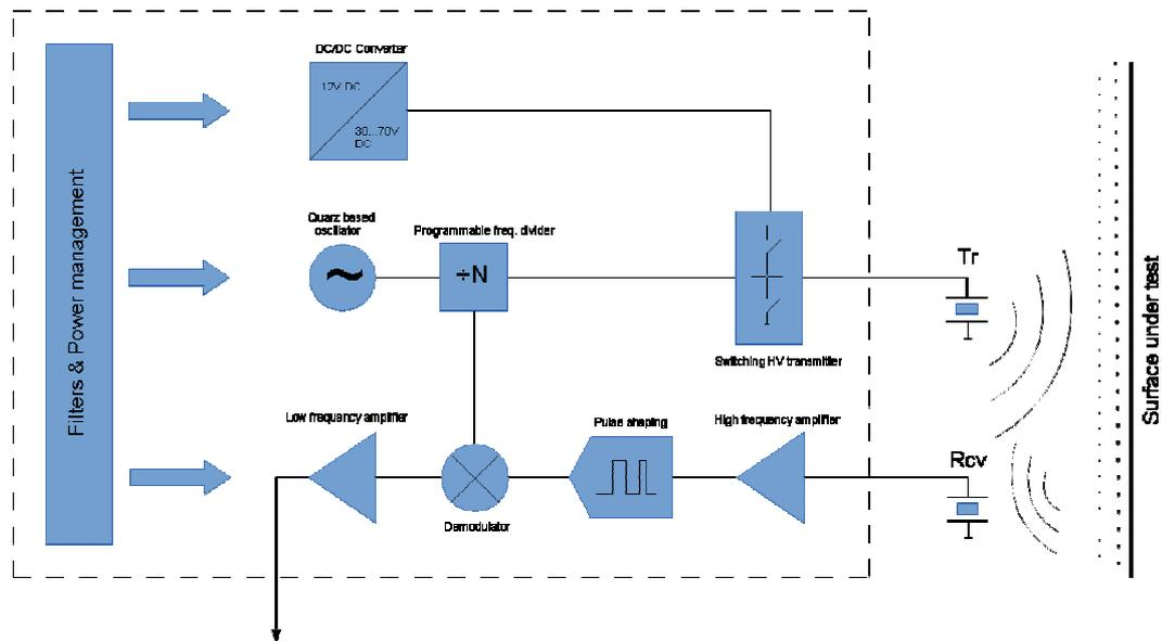
Figure 2. Block diagram of device
